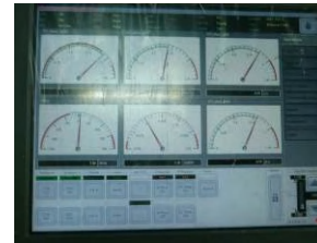
Digital monitor of new exciter system
