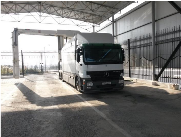
Large truck-mounted X-ray Scanner at Ayritom, at Uzbek-Afghan border. (was out of operation from October 3, 2016 to February 7, 2017. Currently fully in operation.)
