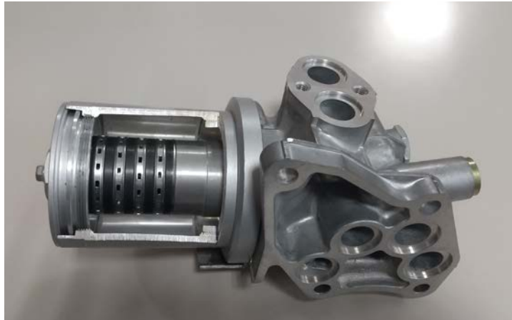
Picture 1 Cross-sectional view of the PECS attached to the engine.
