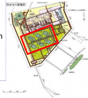
(Yanai Power Plant) Six LNG tanks, each capacity is 80,000kl.
