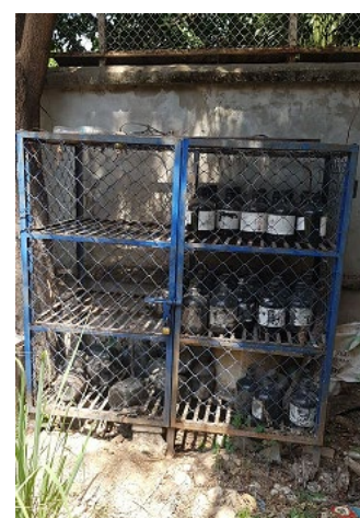
Figure 3-12 Glassware for Outdoor Wastewater Storage (Photograph from NAL)
