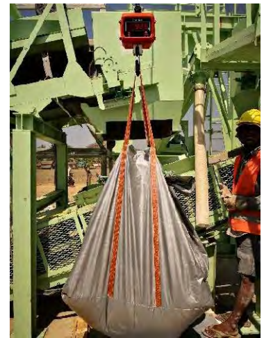
SF to be calibrated at 3 frequency (50Hz @120sec, 65Hz @90sec, 80Hz @75sec) for 3 times
