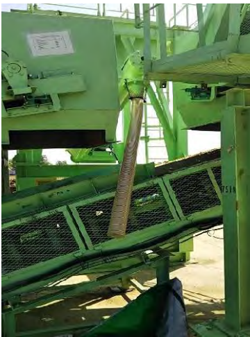
SF to be calibrated at 3 frequency (50Hz @120sec, 65Hz @90sec, 80Hz @75sec) for 3 times
