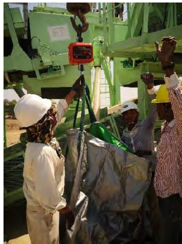
SF to be calibrated at 3 frequency (50Hz @120sec, 65Hz @90sec, 80Hz @75sec) for 3 times
