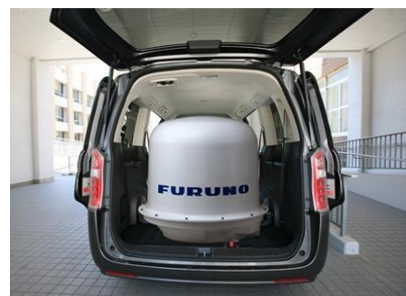
Figure 1 Compact X-band dual-polarization weather radar
