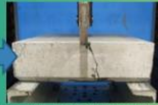
LOADING TEST AFTER CURING
