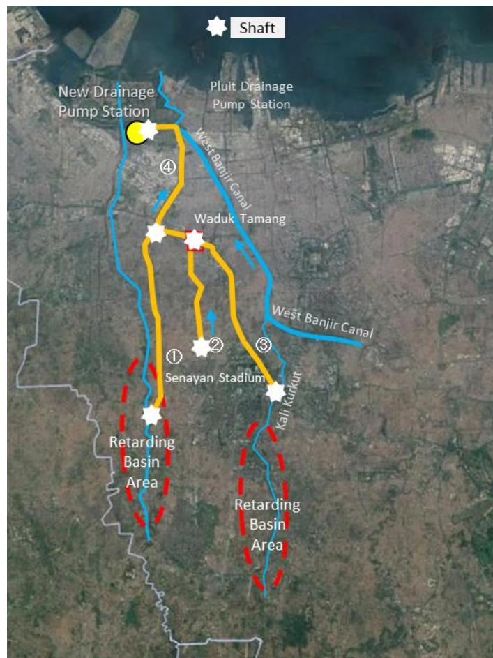
Figure 4-77 Underground Channel Route
