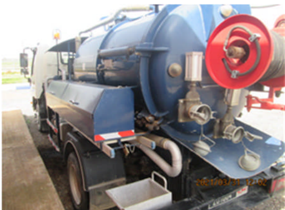
Photo 3: Sewage pipe cleaning equipment (El Kelaa des Sraghna City)
