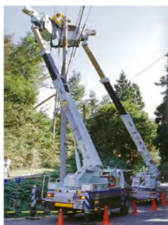
Figure 8.4-2 Comparison of the appearance of a vehicle for distribution work (Top: EDM's current vehicle, Bottom: Japanese product)
