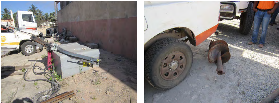
Figure 6.2-17 Bucket (left) and auger (right) to be installed on EDM's truck with crane
