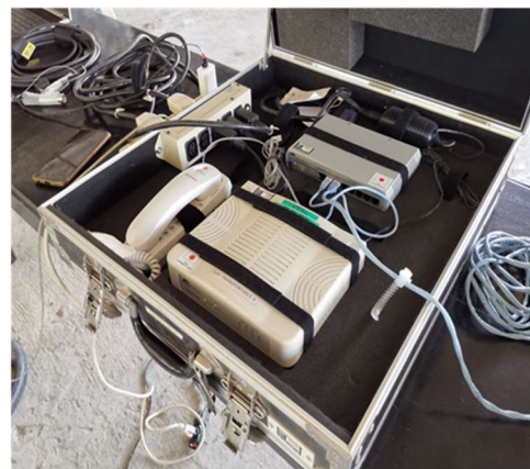
Portable VSAT for emergency use
