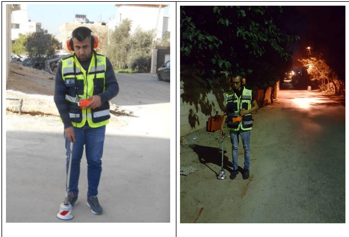
Figure 12-3: Line-Wise Survey Using Ground Microphone
