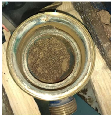
Sand and particles in volumetric meter
