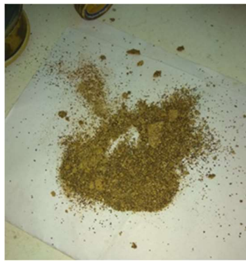
Removed sand and particles from meter
