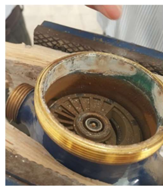
Scale adhered to meter
