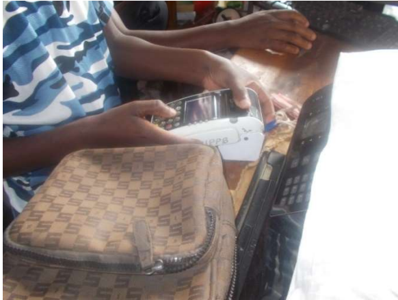
Photo 1. A credit vending machines and a credit vendor. Note the token sticking out at one end of the machine.
