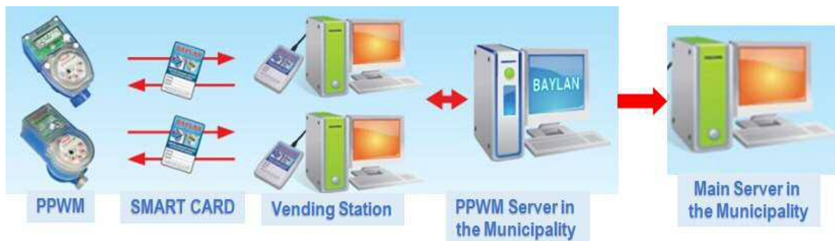
Fig.2.2 Communication flow of Charging Credit
