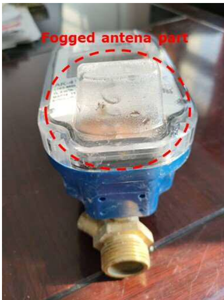
Photo 10.1: Fogged PPWM display due to leakage
