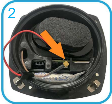
Carefully disconnect the internal antenna
