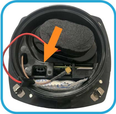
Carefully disconnect the battery cable
