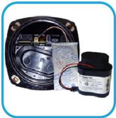
Remove old battery and desiccant pack
