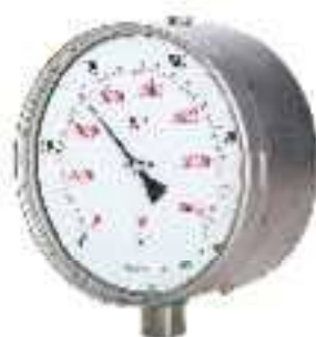
Example of the widely used Bourdon pressure gauge
