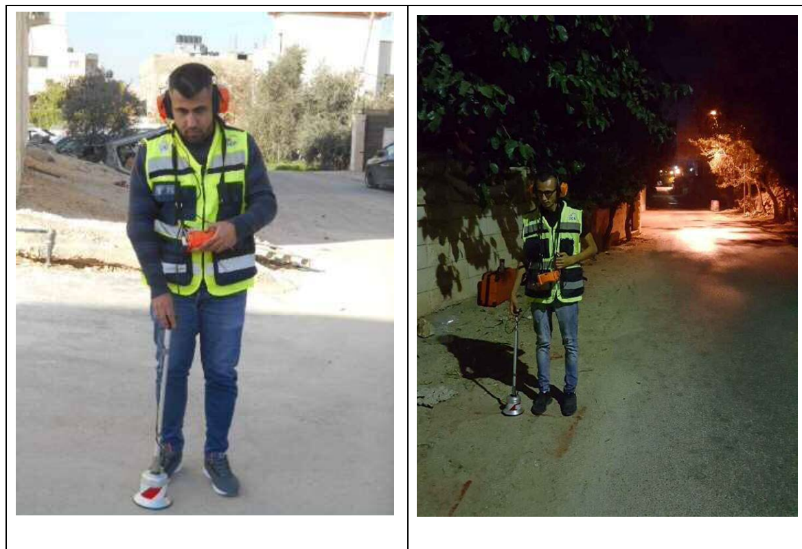
Figure 22: Line-Wise Survey Using Ground Microphone
