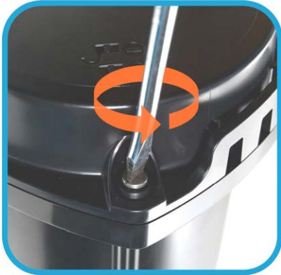
Loosen 4 in no. Camlok screws
