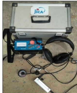
Leakage Detector Provided by this Project
