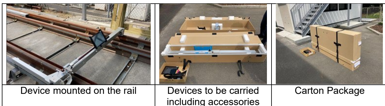
Figure II-6 Geometric Recording Trolley (LR-S100)
