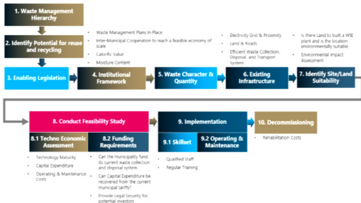
Figure 7-19 Roadmap for Realizing WtE Project
