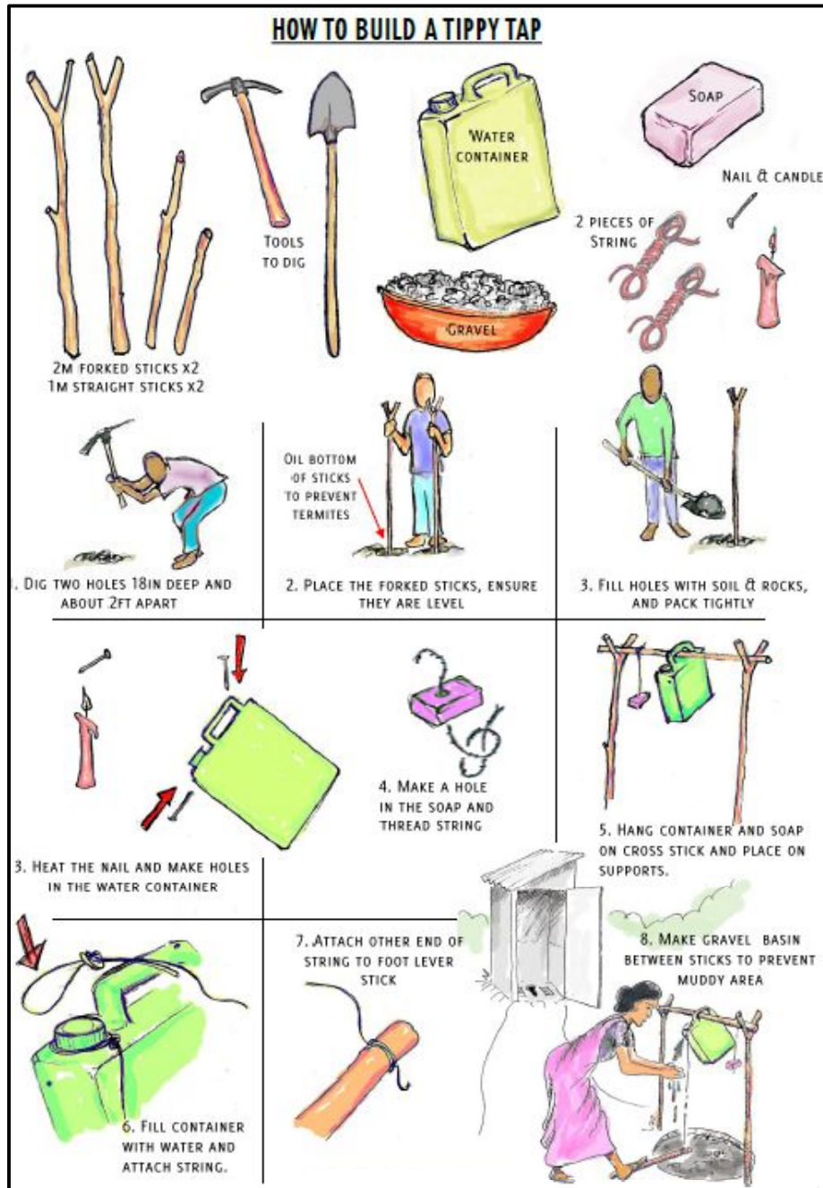
Figure 6: Procedure on construction of a tippy tap (Tippy Tap.org, Watershed Management group, Grampari)
