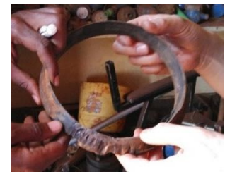
Worn out gasket due to leaking water flow
