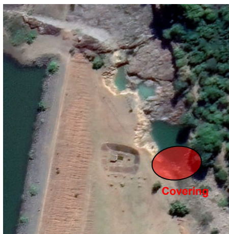
Figure 5.4.3 Outline of Emergency Repairing Measure for Exposure of Siphon Lining Concrete on the Connection Canal Bed
