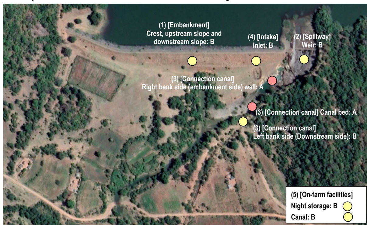
Figure 5.3.1 Locations of Deteriorations/Damages on Magudu Dam
