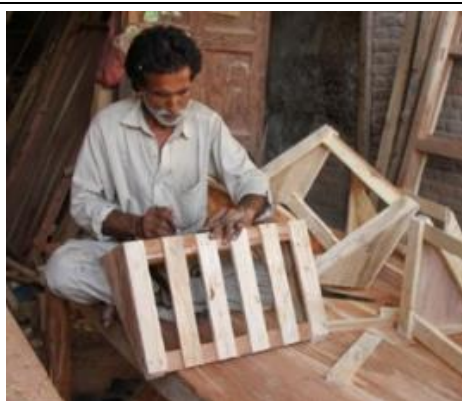
Photo 3-23 Local carpenter making wooden hay rack
