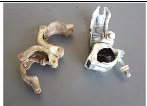
Photo 3-45 Flexible cramp (left) and Fixed cramp (right)
