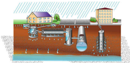
Rainwater Infiltration Well & Trench
