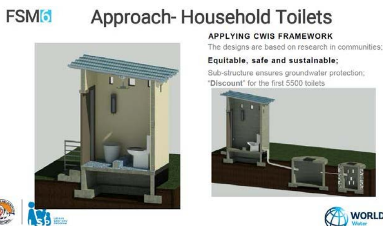
Figure 5-4 Standard Design of Improved Pit Latrine
