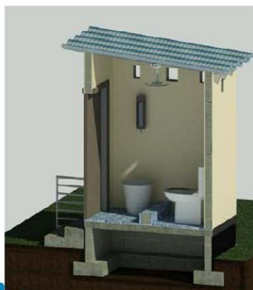
Figure 4-2 Standard Design of Improved Pit Latrine
