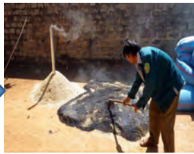
After finish, use water to extinguish when the fire comes out
