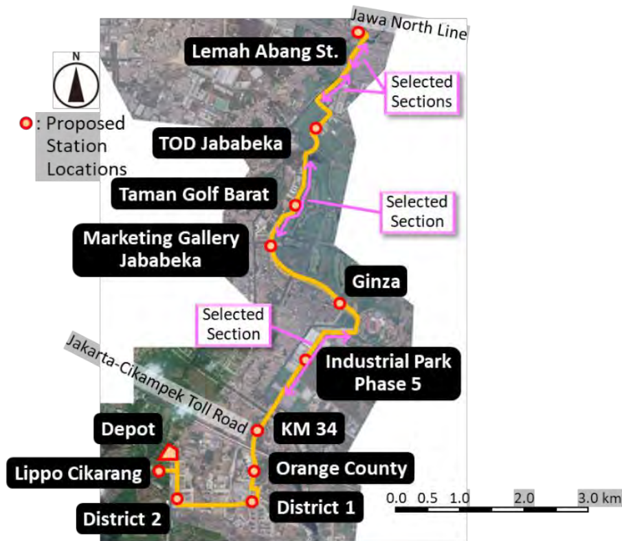
Figure 10-3: Location of the Sections where the Structure Was Changed from Viaduct to Embankment
