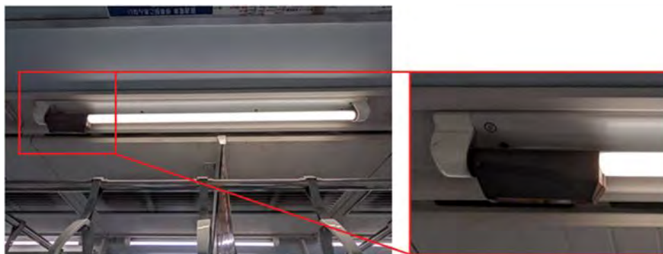
Figure 8-5: Security Camera with Integrated Lighting (With Wireless Communication Function)
