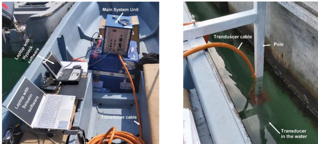
Figure 1-6: Sub-Bottom Profiler (SBP) Equipment Mounted on Research Ship
