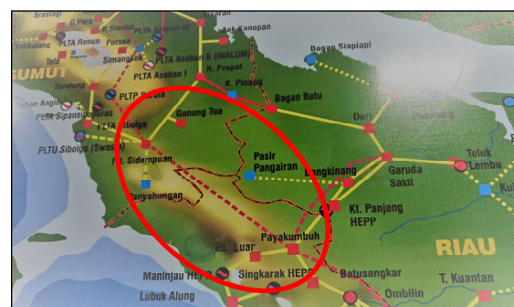
The transmission lines constructed by the project shown in the Sumatra power system diagram
