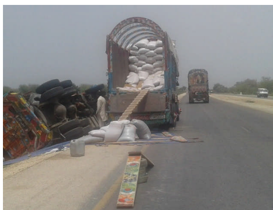
Photo 4: Accident Caused by Overloading
