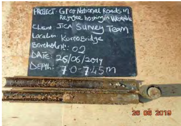
PHOTO 7: Very stiff light orangey grey sandy clay drilled from BH2 (7.0-7.45m), SPT N=19
