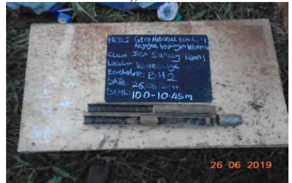
PHOTO 10: Very dense yellowish grey with black patches weathered rock recovered as clayey sand drilled from BH2 (10.0-10.45m), SPT N=52
