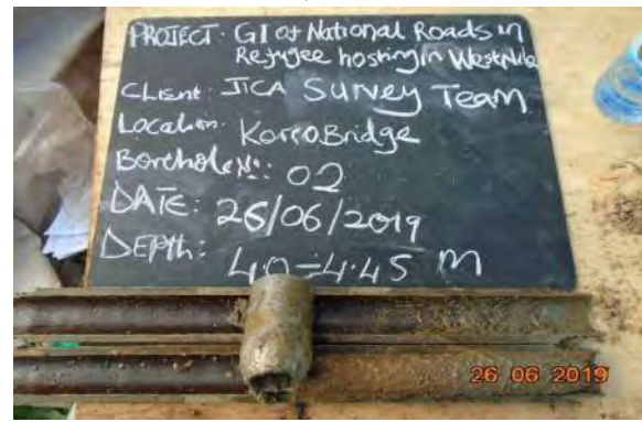
PHOTO 4: Medium dense dark brown moist clayey sand drilled from BH2 (4.0-4.45m), SPT N=12
