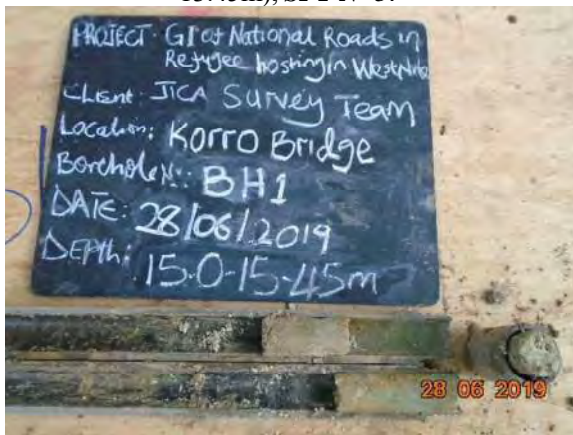
PHOTO 15: Light grey weathered rock (recovered as dense clayey sand) drilled from BH1 (15.0-15.45m), SPT N=59
