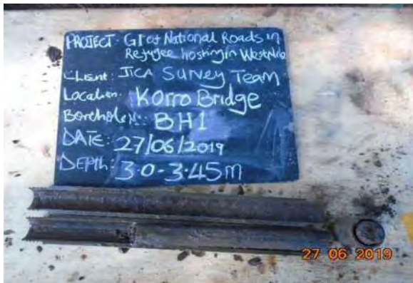
PHOTO 3: Stiff black to dark brown sandy clay drilled from BH1 (3.0-3.45m), SPT N=12
