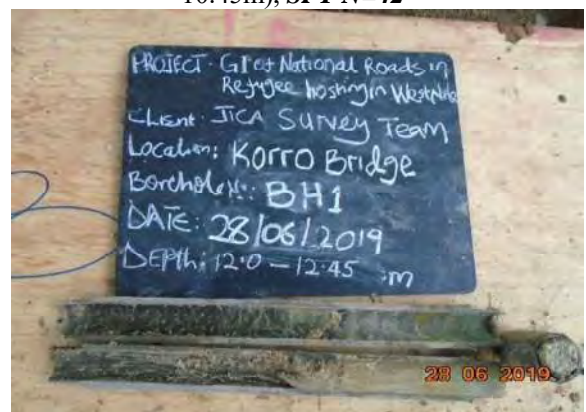
PHOTO 12: Light grey weathered rock (recovered as dense clayey sand) drilled from BH1 (12.0-12.45m), SPT N=55
