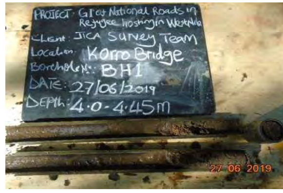
PHOTO 4: Medium dense brown with white patches fine to medium grained moist sandy clay drilled from BH1 (4.0-4.45m), SPT N=16
