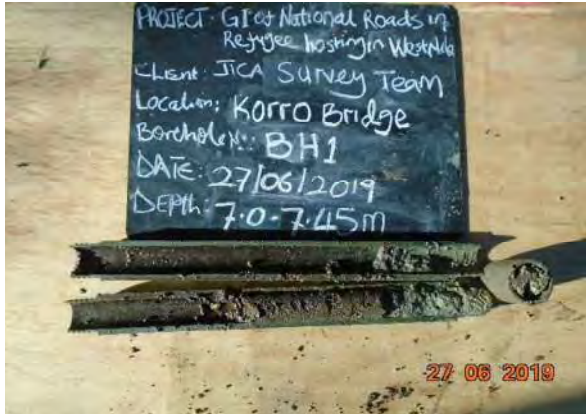
PHOTO 7: Dense brown with white patches fine to medium grained moist clayey sand drilled from BH1 (7.0-7.45m), SPT N=31
