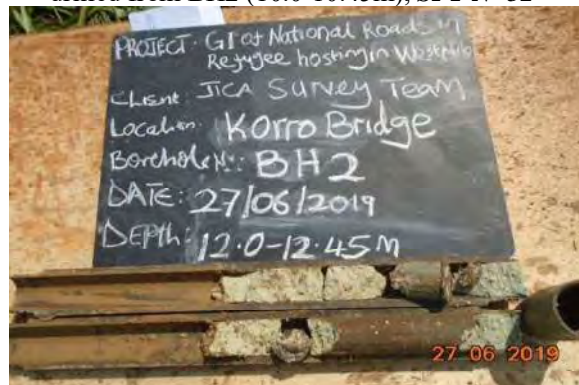
PHOTO 12: Very dense yellowish grey with black patches weathered rock recovered as clayey sand drilled from BH2 (12.0-12.45m), SPT N=54
