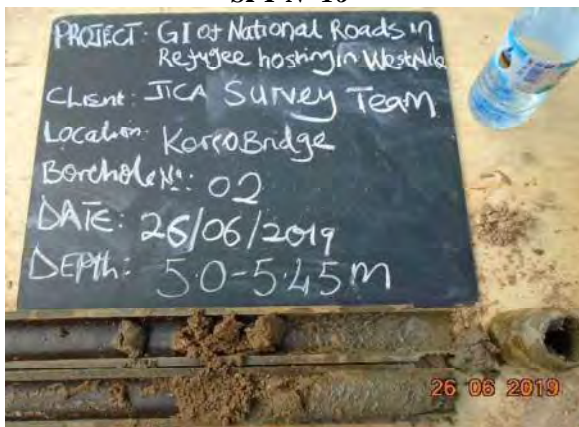
PHOTO 5: Loose brown medium to coarse grained clayey sand drilled from BH2 (5.0-5.45m), SPT N=10
