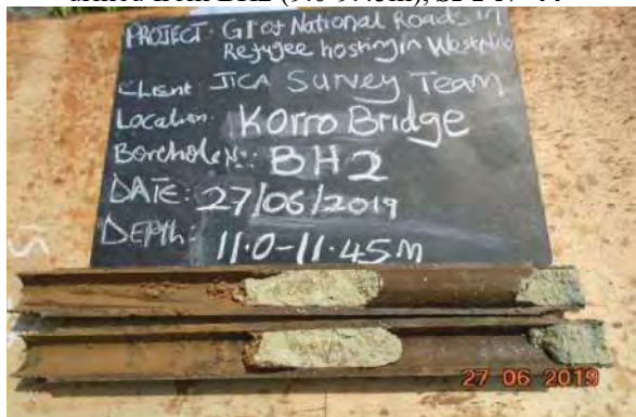
PHOTO 11: Hard yellowish grey with black patches weathered rock recovered as sandy clay drilled from BH2 (11.0-11.45m), SPT N=51
