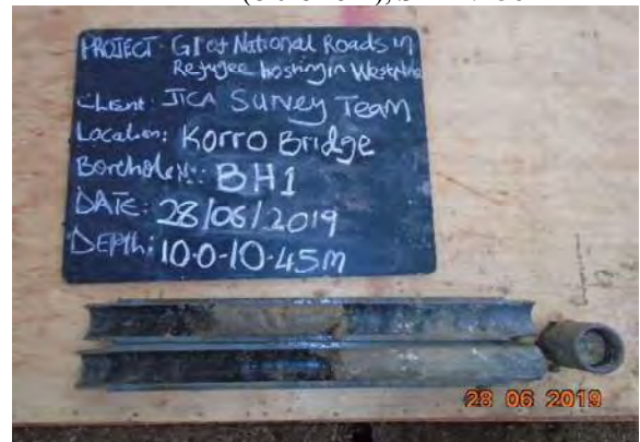
PHOTO 10: Light grey weathered rock (recovered as hard sandy clay) drilled from BH1 (10.0-10.45m), SPT N=42
