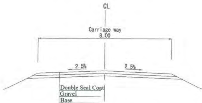
Figure 3-3 Cross Section of approach road (Draft)
