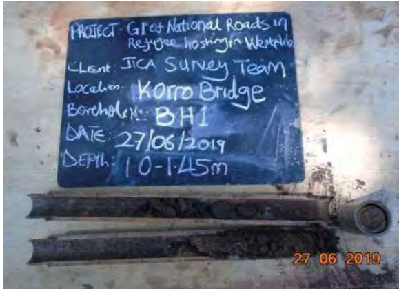
PHOTO 1: Medium dense dark brown organic sand drilled from BH1 (1.0-1.45m), SPT N=19
