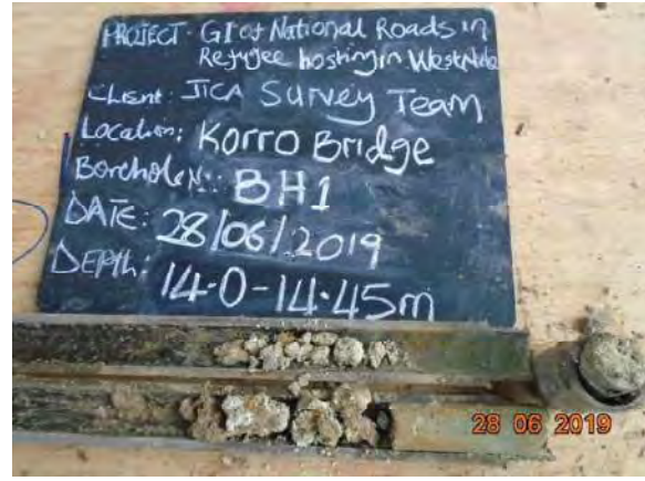
PHOTO 14: Light grey weathered rock (recovered as dense clayey sand) drilled from BH1 (14.0-14.45m), SPT N=58
