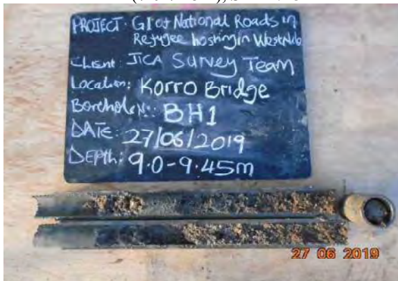
PHOTO 9: Dense Light grey weathered rock (recovered as clayey sand) drilled from BH1 (9.0-9.45m), SPT N=44
