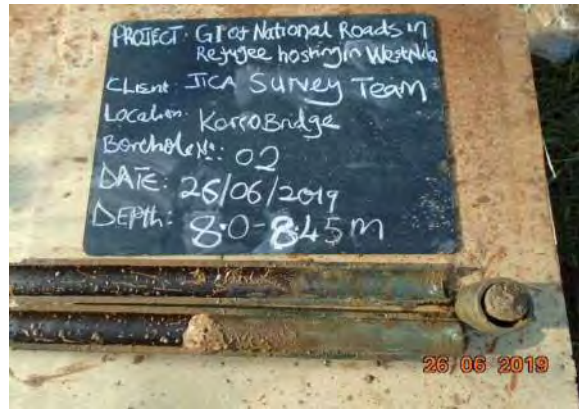
PHOTO 8: Hard yellowish grey weathered rock recovered as sandy clay drilled from BH2 (8.0-8.45m), SPT N=45
