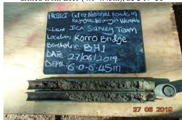
PHOTO 6: Medium dense brown with white patches fine to medium grained moist clayey sand drilled from BH1 (6.0-6.45m), SPT N=22
