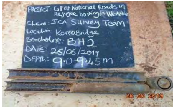
PHOTO 9: Dense yellowish grey with black patches weathered rock recovered as clayey sand drilled from BH2 (9.0-9.45m), SPT N=44
