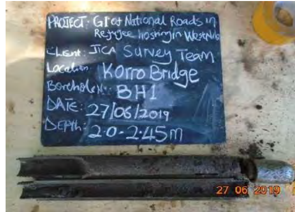
PHOTO 2: Very stiff black to dark brown sandy clay with sand drilled from BH1 (2.0-2.45m), SPT N=17
