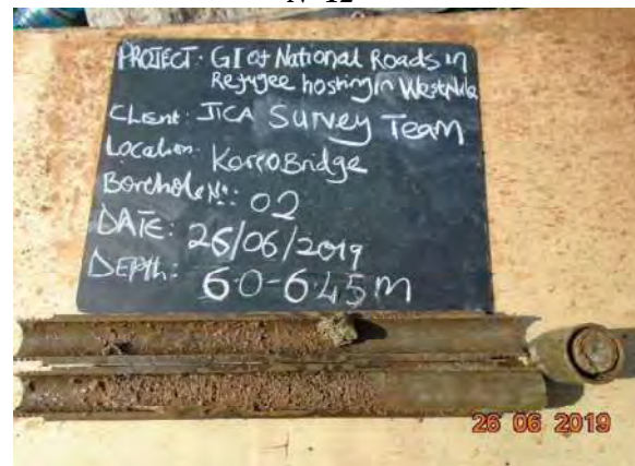
PHOTO 6: Stiff grey sandy clay drilled from BH2 (6.0-6.45m), SPT N=13
