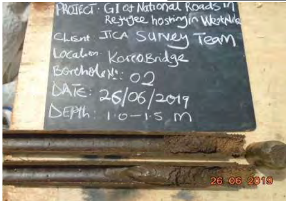
PHOTO 1: Loose organic silty clayey sand drilled from BH2 (1.0-1.45m), SPT N=8
