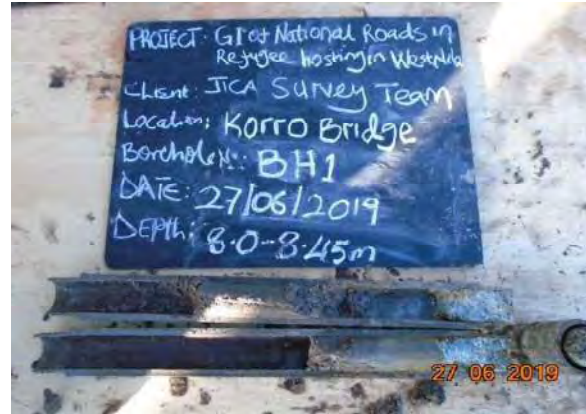
PHOTO 8: Dense light grey with orangey patches clayey sand turning into weathered rock drilled from BH1 (8.0-8.45m), SPT N=36
