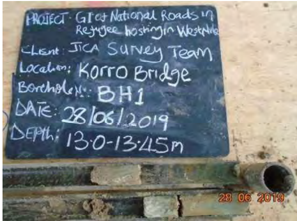
PHOTO 13: Light grey weathered rock (recovered as dense clayey sand) drilled from BH1 (13.0-13.45m), SPT N=57
