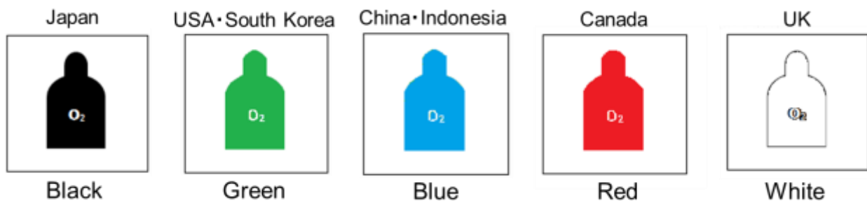
Figure : Colors of imported oxygen cylinder in Myanmar
