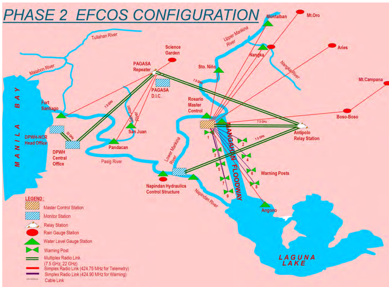
Figure 3.2.10 Improved System Configuration of EFCOS (Phase 2)
