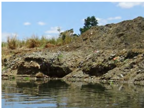
Figure 5.2.9 (Photo) Cohesive soil layer on the left bank of the Lower Marikina River
