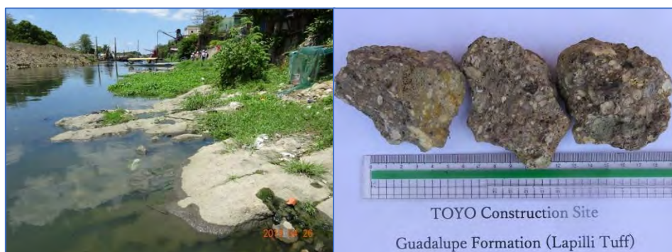
Figure 5.2.6 (Photo) Guadalupe Formation along the C5 Highway (Lapilli tuff)
