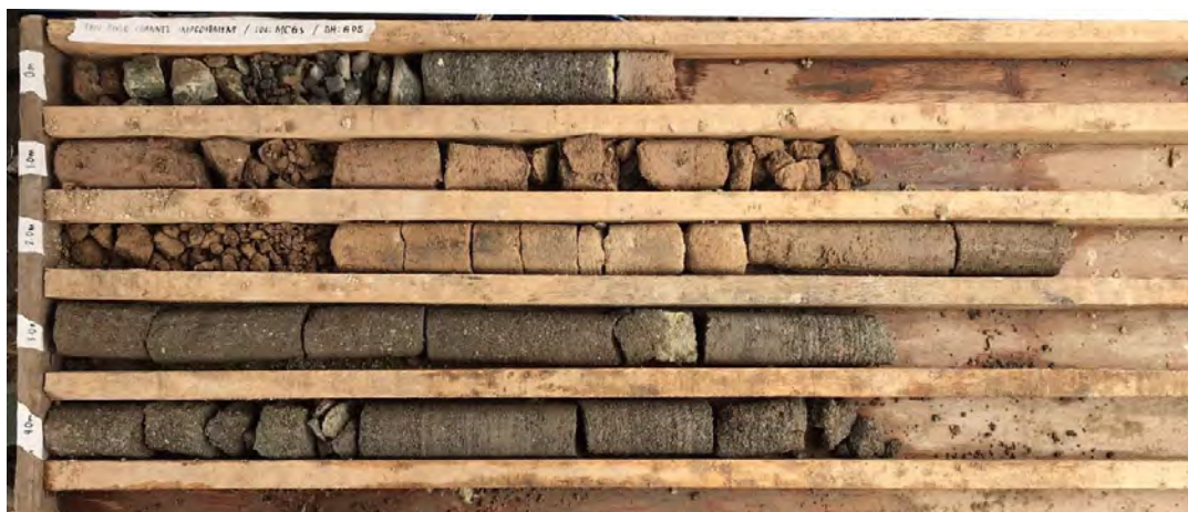
Figure 5.2.17 (Photo) 0-5m core of BH-G-05 hole (Red part is tuff gray part is lapilli tuff)
