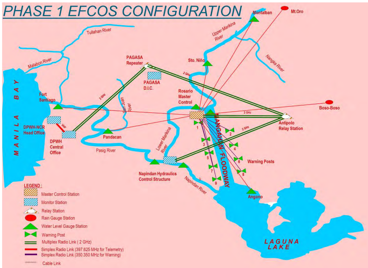
Figure 3.2.9 System Configuration of EFCOS (Phase 1)
