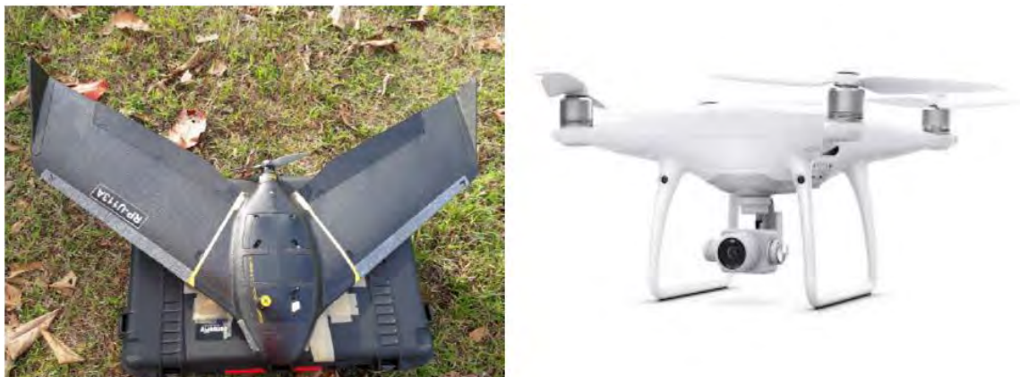
Figure 5.1.6 Aircrafts used for Aerial Survey (Left: Sensefly eBee X, Right: Phantom 4 Pro v2)
