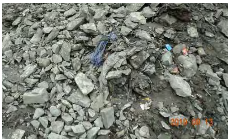
Figure 5.2.19 (Photo) Excavated rock composed of fresh tuff
