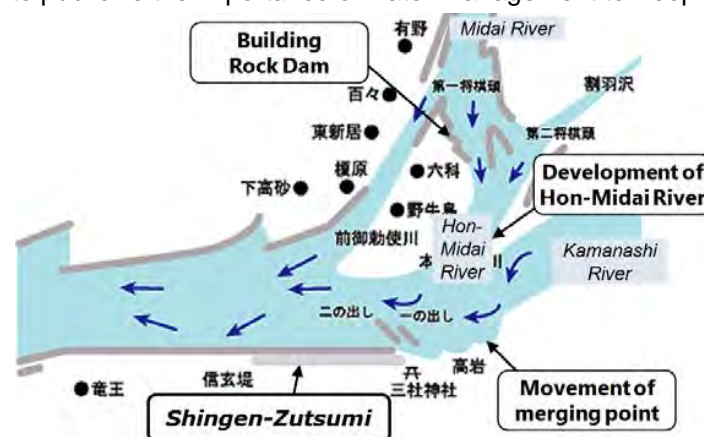
Fig. 6-8: Outline of Shingen-Zutsumi (Source: MLIT) 62
