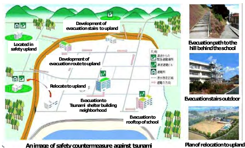
Fig. 6-2: Example of structural measures against Tsunami in Schools 49 (Source: MEXT)
