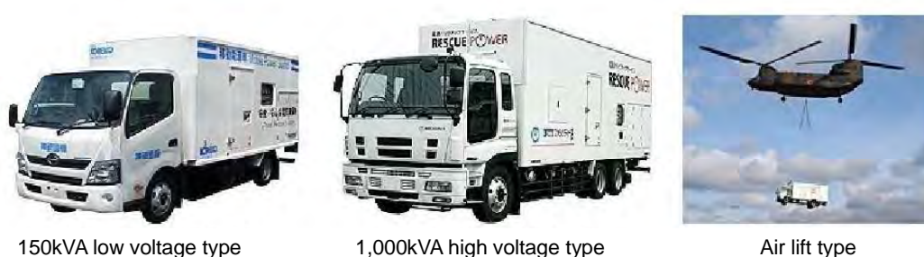
Fig. 6-32: Generator vehicles (Source: Shinko Zoki Co., Ltd.)
