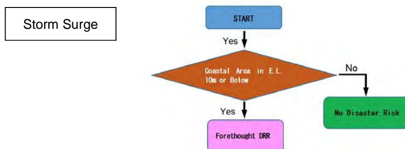
Fig. 4-5(3): Procedure of screening with hazard and topography data.
