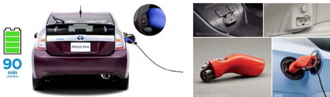
Fig. 6-41: Toyota Prius PHV with equipment of 100V power outlets (ZVW 35, JDM model)
