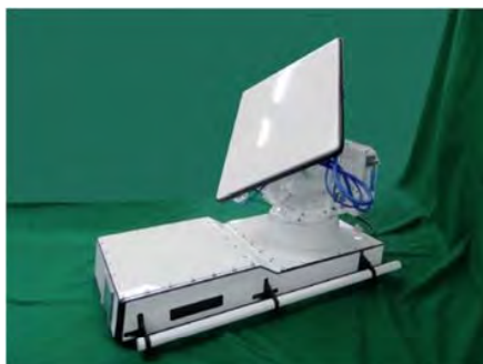
Fig. 6-29: Prototype VSAT (Source: SKY Perfect JSAT Corporation)
