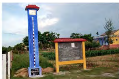
They are examples of approach for regional disaster management by village people. Two facilities had been installed; the water level pole to measure the extent of the flood and bulletin board for and information sharing.
