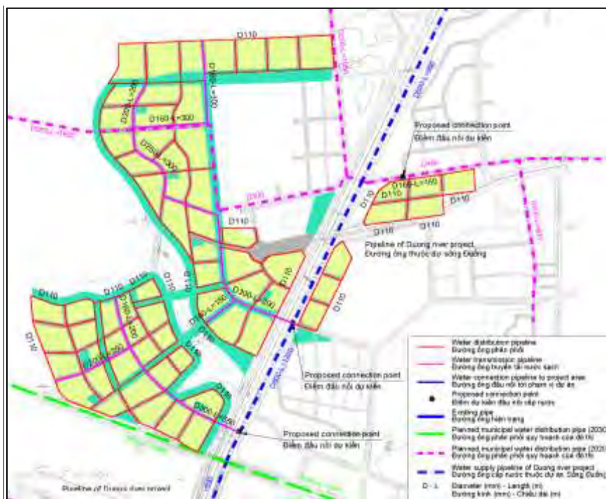
Figure 16-19. Layout of Water Supply Network (region N3)
