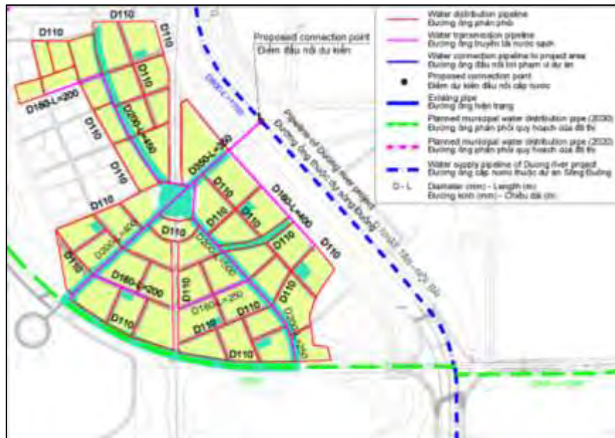
Figure 16-22. Layout of Water supply network (region N6)
