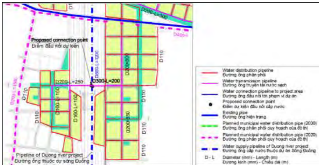
Figure 16-21. Layout of Water Supply Network (region N5)
