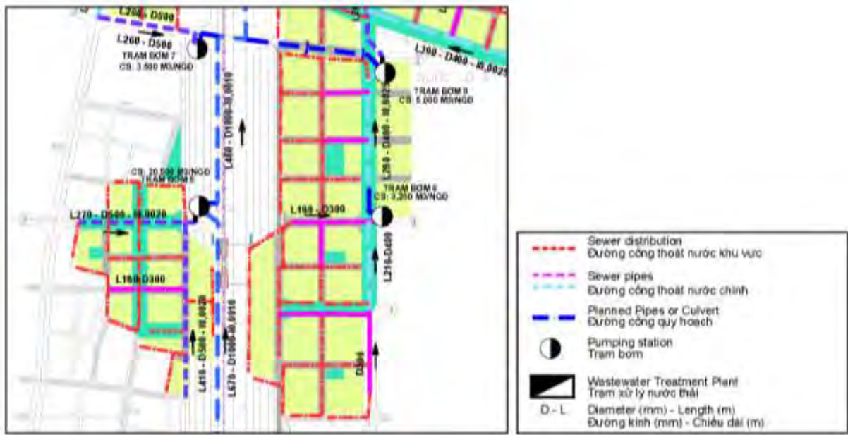
Figure 16-28. Layout of Sewerage System (region N5)
