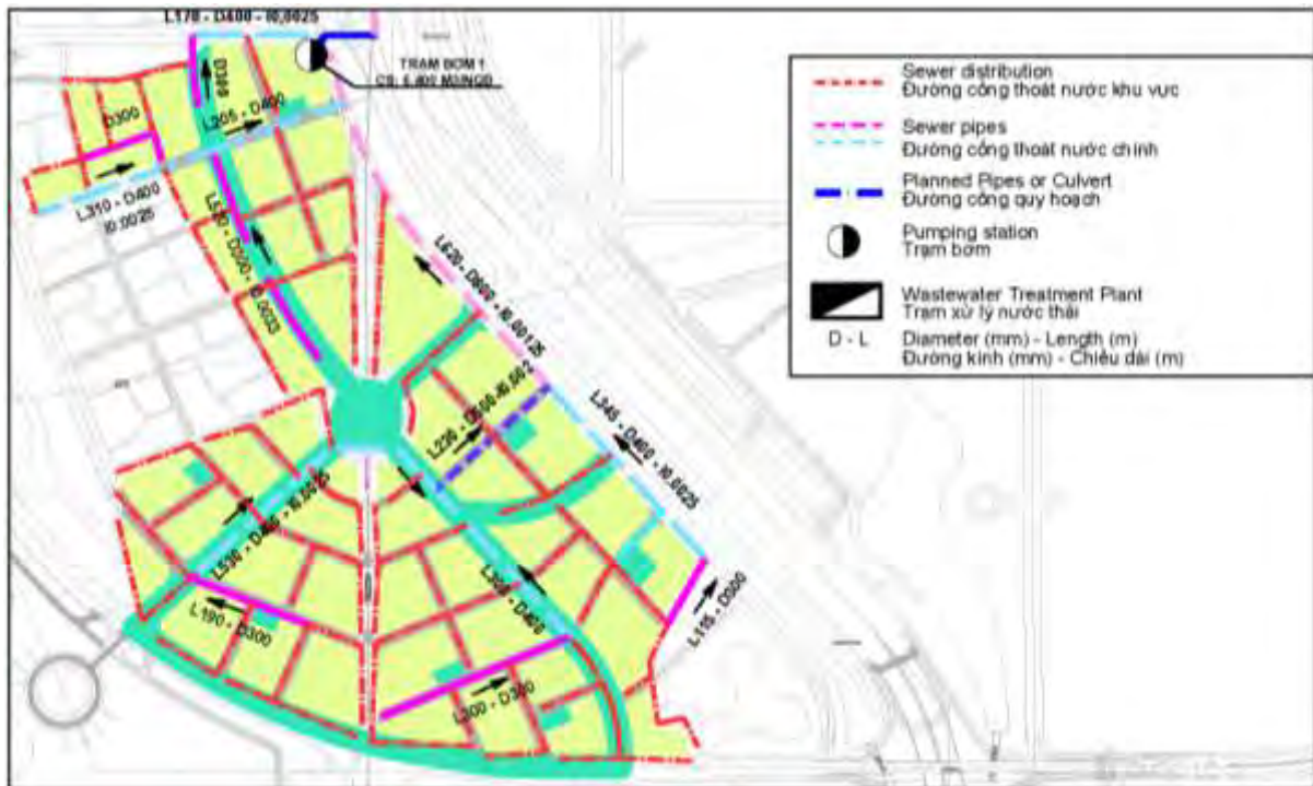
Figure 16-29. Layout of Sewerage System (region N6)
