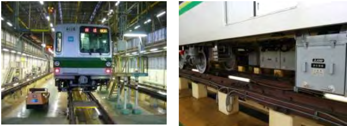
Figure 9-20. Inspection and Repair Tracks
