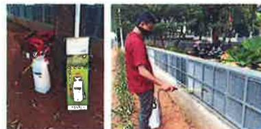
ACF was washed by a little amount of water (8L) before measurement in the 4<sup>th</sup> period on 26 ~ 30 August 2019. The NO2 removal was regenerated obviously compared to July.
