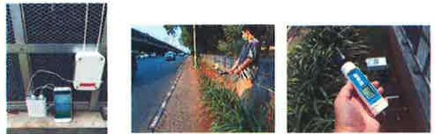
PM2.5 Monitor      SO<sub>2</sub> sampling tube      CO Monitor
