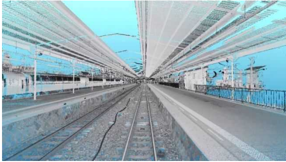
Figure 3 Left: An example of using 3D point cloud data by the railway version of InfraDoctor/ Right: measurement by the airport version of InfraDoctor.
