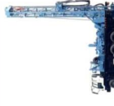
Truck mounted Water well drilling Machine
