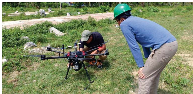
Figure 10. Yellowscan mounted on DJI Matrice 600
