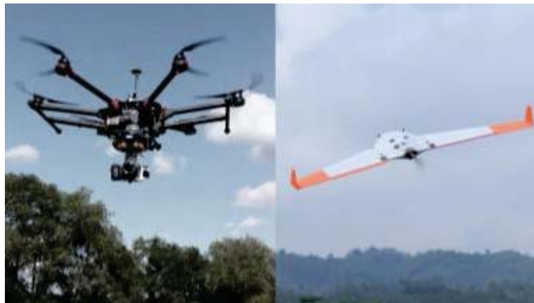
Figure 3. Drone type Multirotor (left), and Fixed Wing (right)
