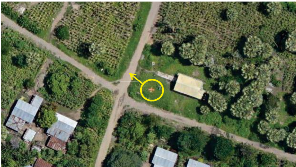
Picture 5. Example of GCP in one of aerial photos
