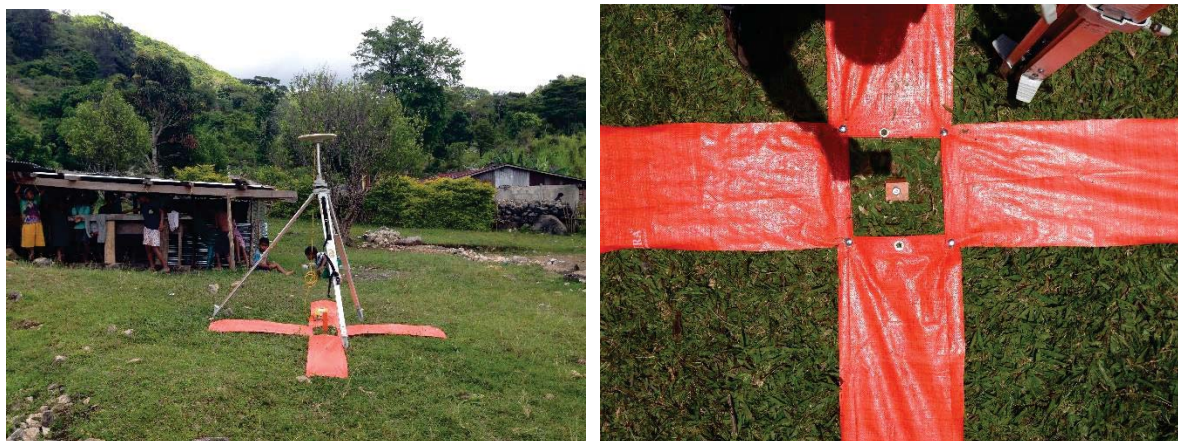
Picture 19. Sample of GCP Measurement and Premark Installment
