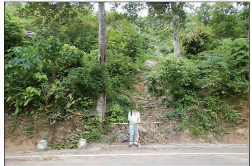
P4 Trace of the surface flow, which removed the sediments around the huge boulders and thus promoted instability
