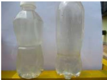
**Fig.3-21 Appearance of sludge in bottles (Left: Inlet, Right: Outlet)**
