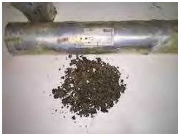
Figure 8. Undisturbed sample of Nampula Central at 5.0m
