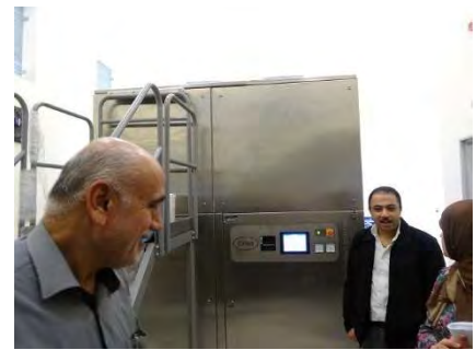
Autoclave for infectious waste treatment
