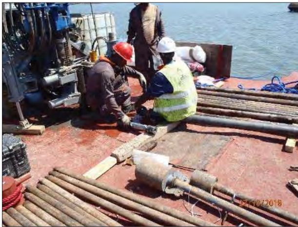
Photography 18 : Recovery of samples in the carrot
