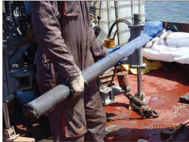
Photography 18 : Recovery of samples in the carrot
