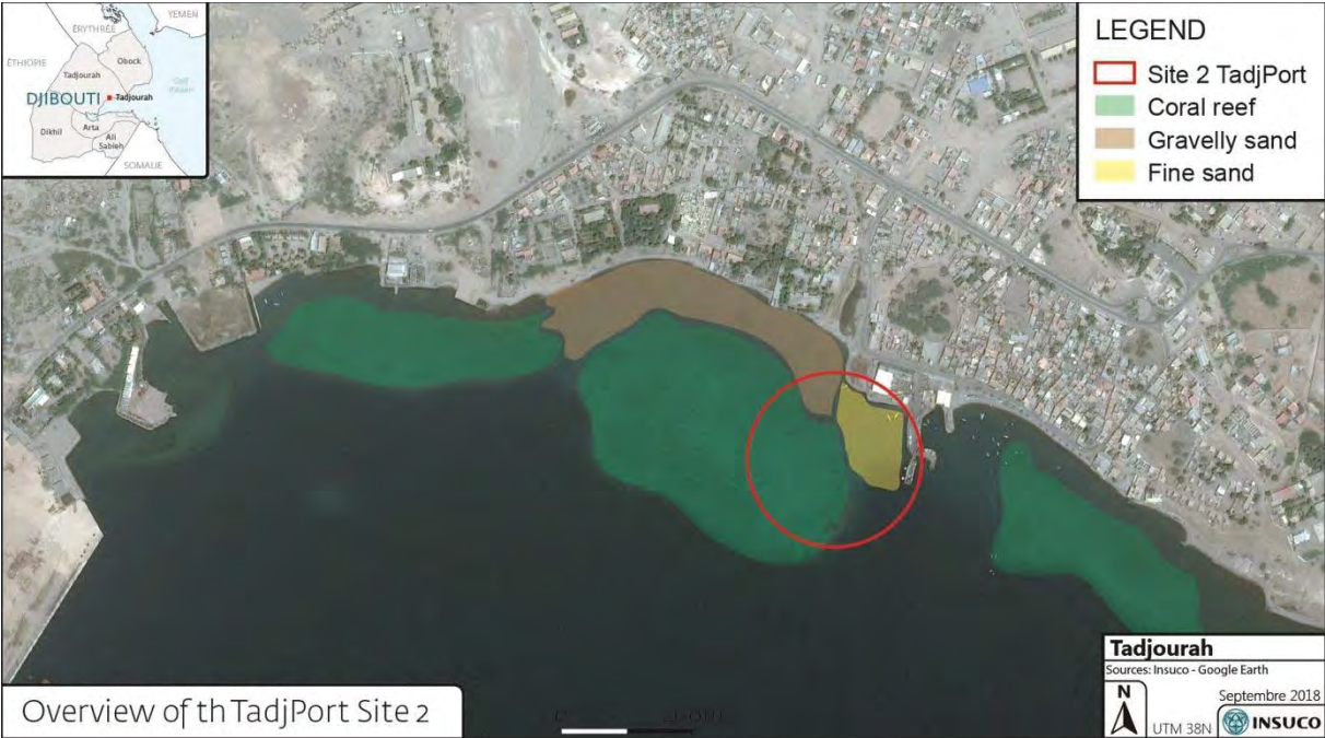
Figure 27 : An overview of the Tadjourah Port -Site -2 showing coral reef, sandy and gravelly seabed
