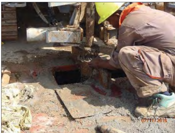
Photography 16: Sediments out of tubing during carotage
