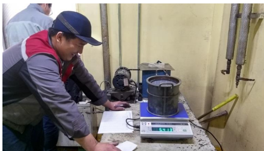
Figure 8 Daily Filter Weight Measurement in order to Calculate PM Weight Collected
