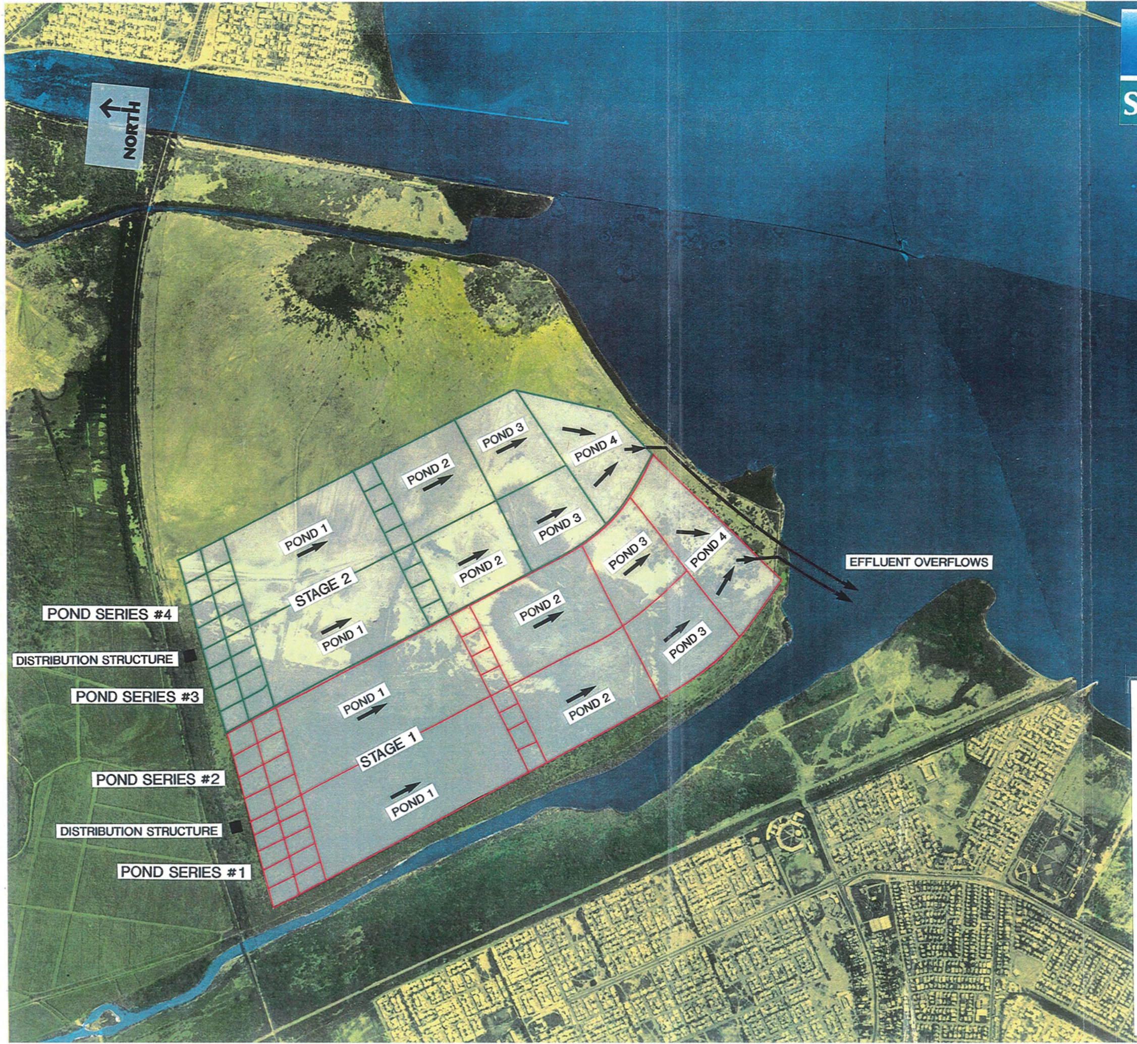
FIGURE XIII.4 KINGSTON HARBOUR ENVIRONMENTAL PROJECT Lagoon Layout Plan (for trial #2)
