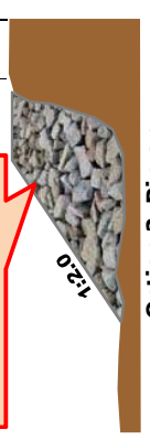
Option-2: Riprap (Dumping Boulder/Gravel)
