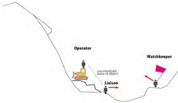
Recommended Avalanche Observation Arrangement
