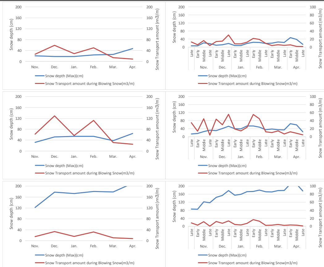
Figure 9-7 Relation between Snow Depth, Snow Transport Amount and Elapse (Too-Ashuu Pass, Upper:A, Middle:B, Bottom:C)
