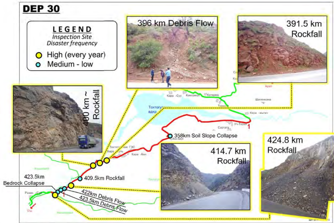
Figure 6-7 Location of Site Reconnaissance in DEU 30
