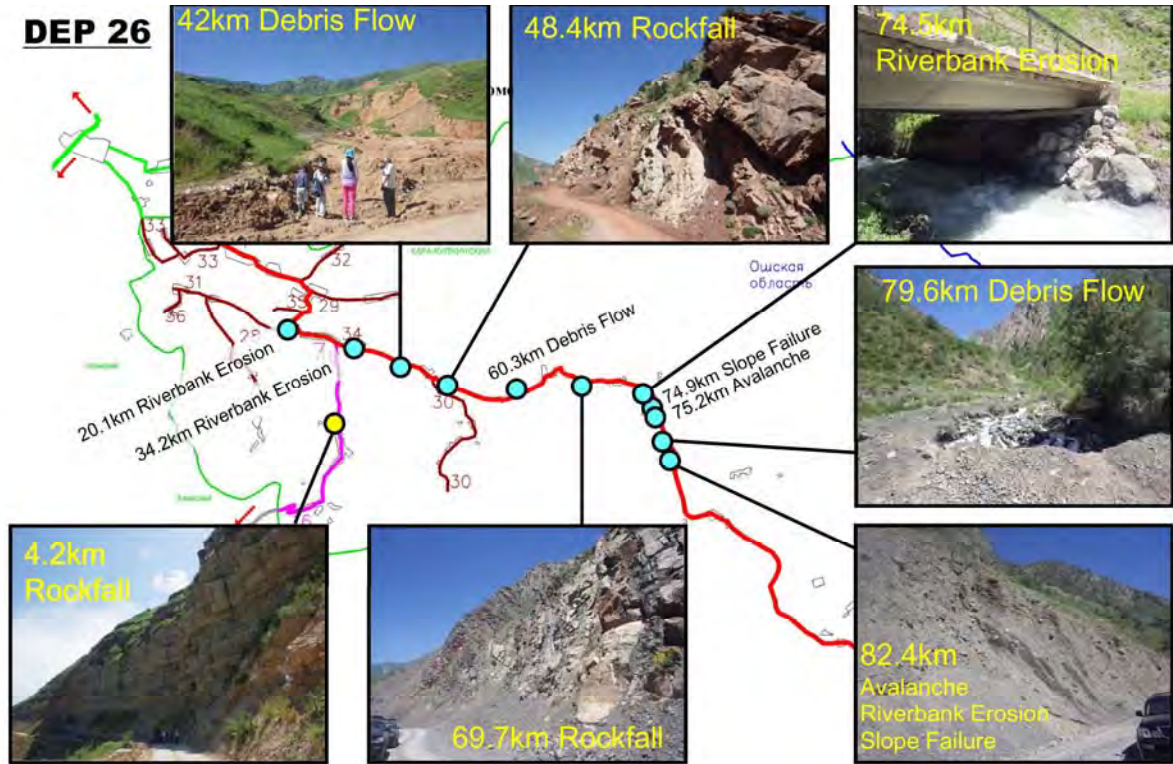
Figure 6-9 Location of Site Reconnaissance in DEU 26
