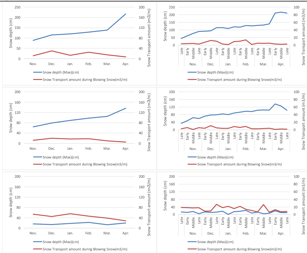
Figure 9-11 Relation between Snow Depth, Snow Transport Amount and Elapse (Ala-Bel Pass, Upper:A, Middle:B, Bottom:C)
